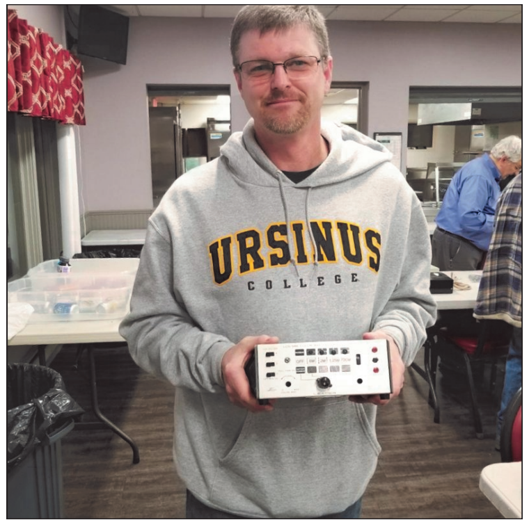
Lee recycled the case from an old NTSC Bar / Dot generator to house his homemade I.F and Keyline selector.
